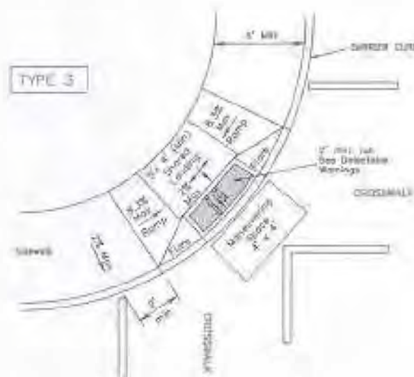
DIAGONAL COMBINATION CURB RAMP Perpendicular to the Tangent of the Curb Radius and Contained in Crosswalk
