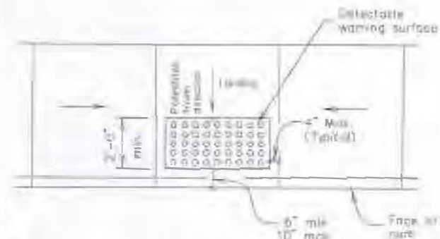
Typical placement of detectable warning surface on landing at street edge.
